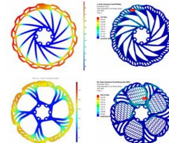
Heat transfer within the design concepts was studied extensively using engineering simulation software. The relationships between convection, radiation, surface area and weight were used to determine the optimal design to maximize heat dissipation and strength while minimizing weight.
