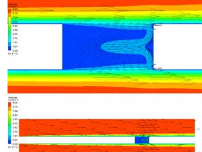
Computational fluid dynamics (CFD) simulations were performed to study airflow over the surface of the rotor and through the cutouts. A variety of profiles were tested to determine the effects of asymmetrical holes and optimize the cooling effect of airflow over the surfaces.
