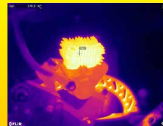
Brake system temperatures are dramatically lower than standard pads, reducing wear on pads and rotors. Lower temperatures also mean more consistent brake performance by reducing brake fade - the reduction of brake power caused by overheated components.
