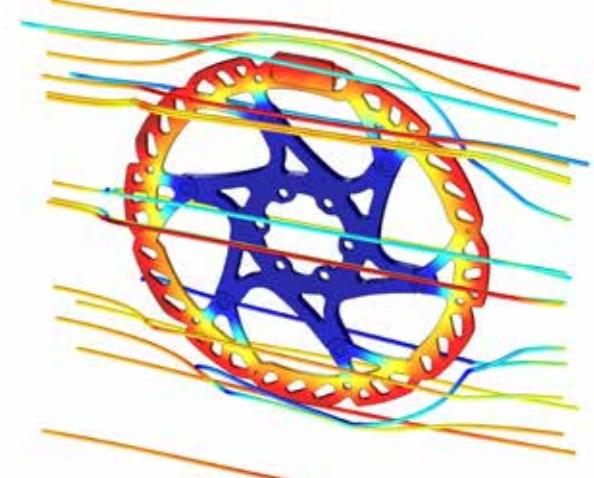
The final design was confirmed and visualized with further thermal and structural simulations.
