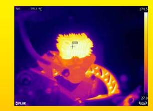
With EXOTherm2 brake system temperatures are dramatically lower than standard pads, reducing wear on pads and rotors. Lower temperatures also mean more consistent brake performance by reducing brake fade - the reduction of brake power caused by overheated
